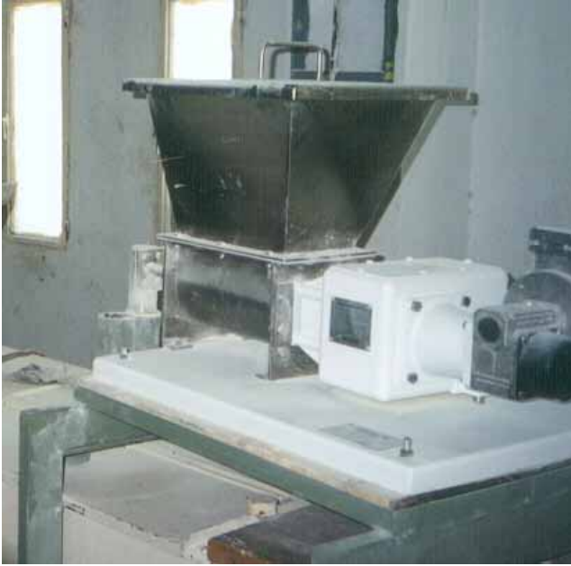
The volumetric feeder is equipped with a screw discharge and is placed directly on top of the flour collection conveyor in a mill in Jordan.
