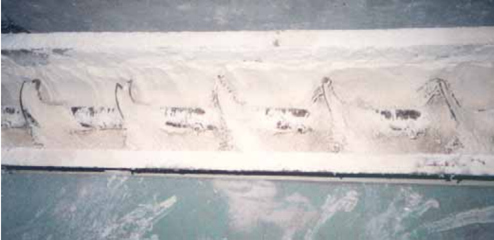
The inside of a flour collection conveyor showing the flight blades of the screw moving the flour along the conveyor. The mill is in India.
